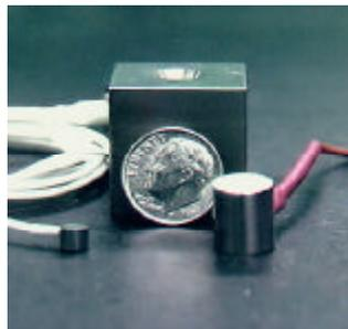
**Figure 11. Acoustic emission sensors**
