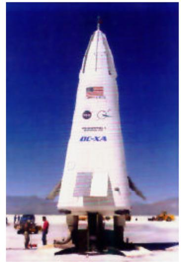
**Figure 8. DC-XA technology demonstrator rocket**
