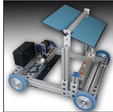
Figure 1. THELIS-P (Thermography Line Inspection System -Portable), developed to use the LST<sup>™</sup> technique to inspect several feet of flat laminate composite samples.
